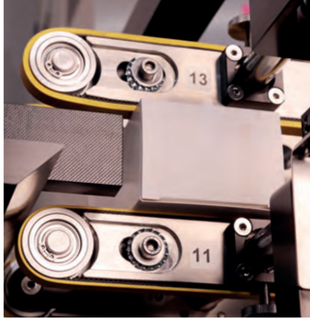
Stable transfer positioning of folding boxes for best print results
