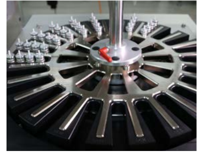
Easy assembly and disassembly of the rotary star wheel
